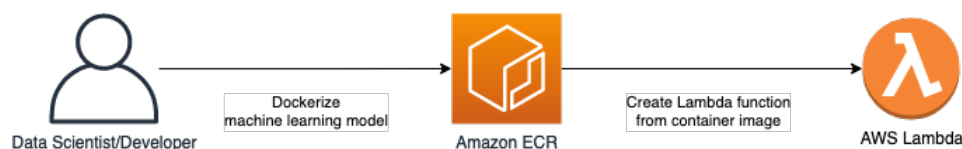
Figure 4.5: AWS architecture of ECR with lambda.
